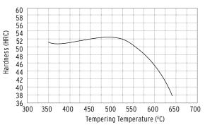
Specimens with cross section of 20 x 20 mm², Tempering time : 2 hr
