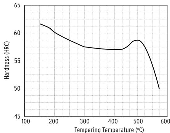
Tempering temperatures should be suitable to the required hardness. If hardness around 60 HRC is necessary, tempering in low temperatures should be employed. However, if 58 HRC or less are possible, tempering at 500°C or higher is preferable, in order to improve toughness. Double tempering is required and after each tool must cool down to room temperature. After soaking, holding time of at least 2 hours is necessary.
